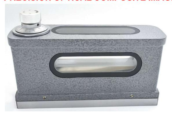
Mainly consists of the micrometer measuring screw, lever systems, standards, optical prisms and a V-shaped base composition working plane
